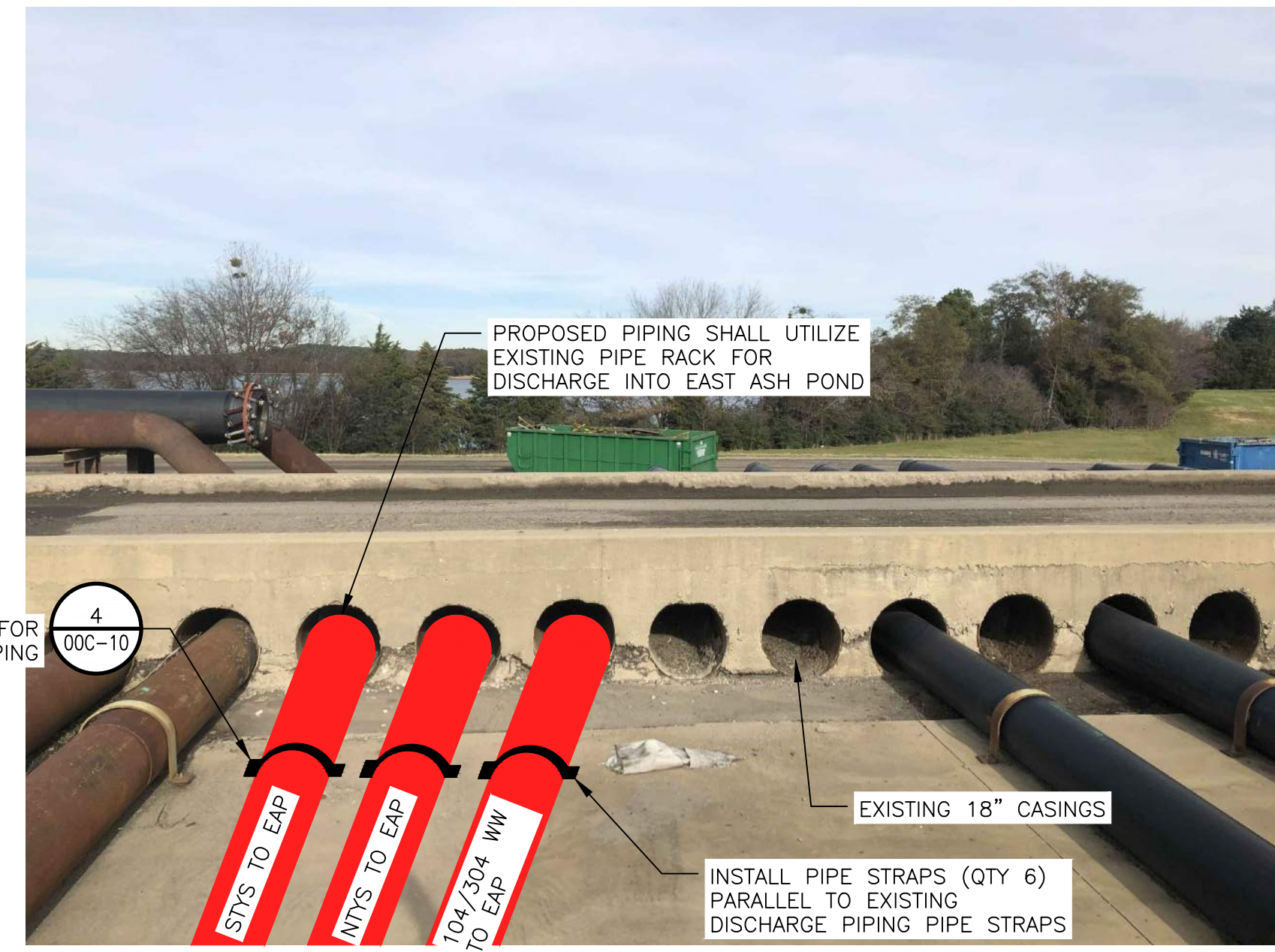
TERMINATION DETAIL A AT EXISTING PIPE RACK (A) NOT TO SCALE 00C-08
